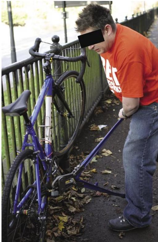
Snip! With 36-inch bolt croppers, the lock above lasted less than 2 seconds. The one opposite lasted 10.6 seconds to mere cable cutters
